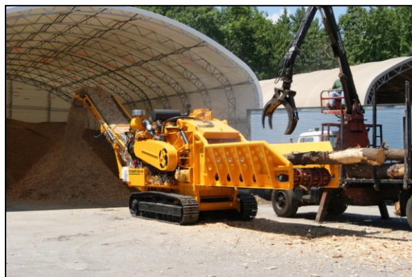
Figure 23. Continental Biomass Industries, Inc. 5800T Grinder. Picture courtesy of CBI, Inc.
