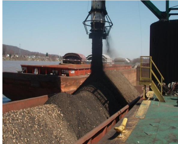
Switchgrass pellets on barge mixed with coal
