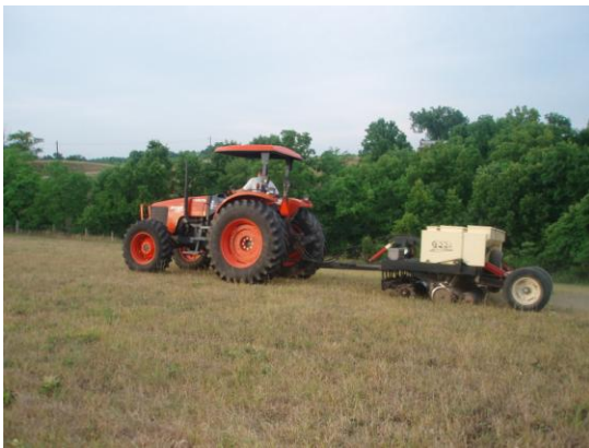
Seeding switchgrass with a no-till drill
